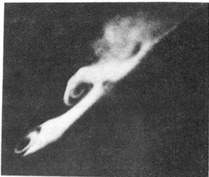
Fig. 27 Cross section of spiral vortices (Kohama and Kobayashi, 1983b). D = 250 mm; N = 1500 rpm.
