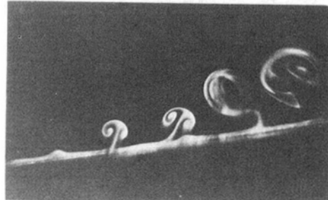
Fig. 10 Cross-sectional flow structure of spiral vortices (Kobayashi and Izumi, 1983). 2\theta = 30 deg.
