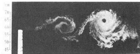
Fig. 9(a) Picture of tip vortex. Without tip vane on the blade tip. By smoke line method.
